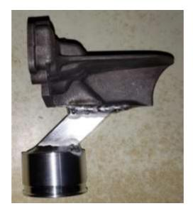
Once you have both ends completely welded, check for leaks. Don't bugger up your sealing surface. It's definitely a good idea to clean the sealing surface and true it up once you're finished welding.
