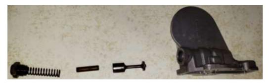
Once you remove the check valve, more oil will present itself. Use non-chlorinated brake parts cleaner to finish cleaning out the housing. The next step is to cut off the bottom portion of the housing. Cut along the line left by the casting mold. Keep your cut parallel with the upper gusset.
