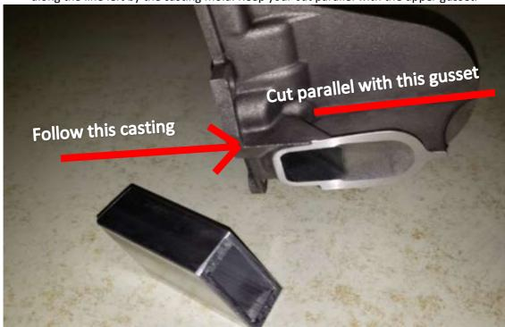
A rear clerance sump pan will require the pick-up to be pointed towards the front of the engine, as shown in the picture, below. Front clearance pans, as used in Jeep YJ's, will require the oposite.
