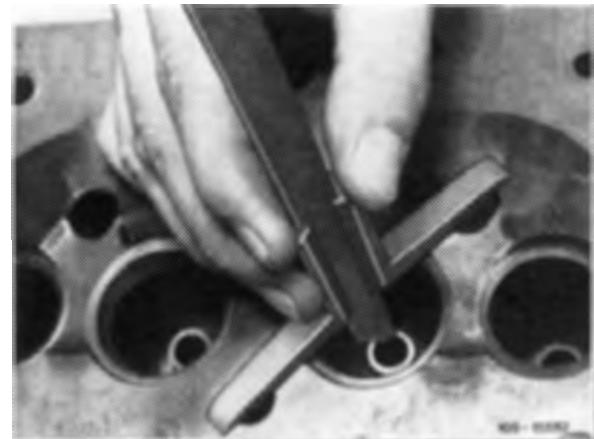
8 Check ID of valve guide with plug gage.
