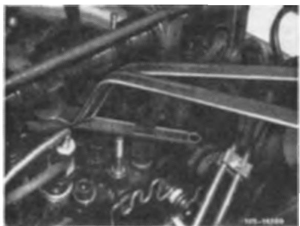
5 Screw dial gage holder with threaded sleeve to stud at front right.
