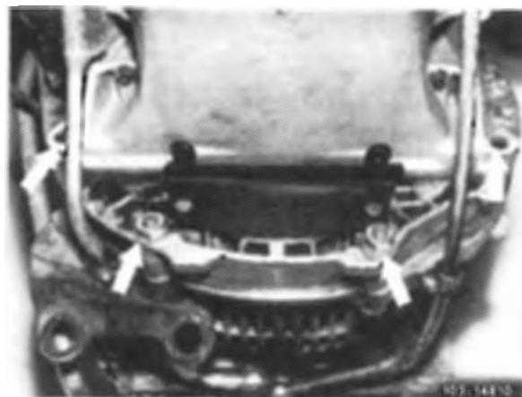
15 Knock-out oil dipstick guide tube as far as possible by means of knocking-out mandrel 9 mm dia. for valve guides.
