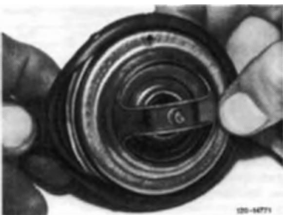
7 Install coolant thermostat with seal in such a manner that arrow on thermostat points upwards.
