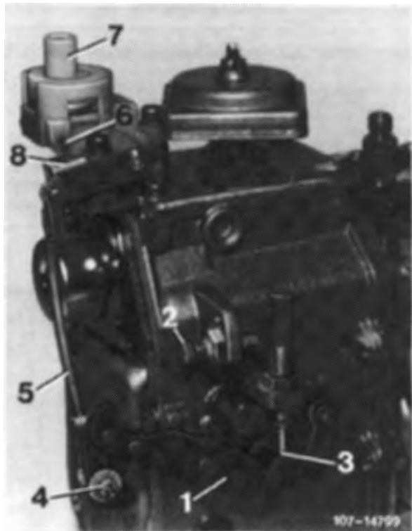
3 Unscrew injection line for cylinder 1.
