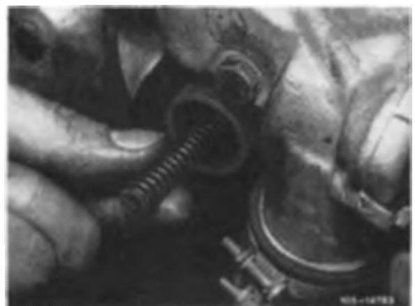
11 Remove slide rail in cylinder head. Pull out bearing bolt by means of impact puller.
