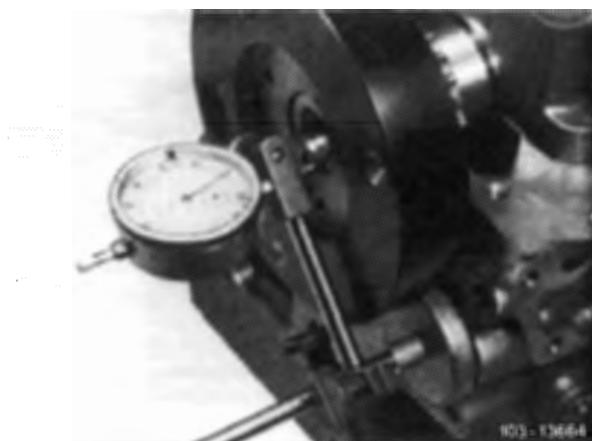
**Coordinating connecting rod bearings and installing connecting rods**
