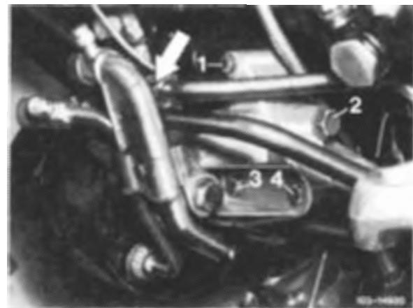
8 Unscrew both engine shock-absorbers on frame cross member or console for lower control arm.
