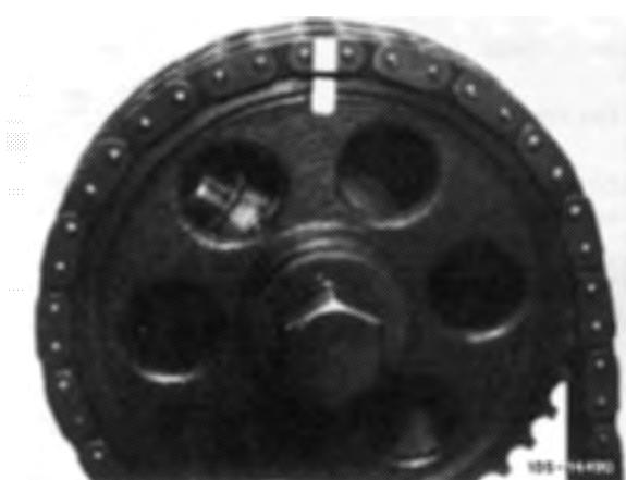
8 Remove camshaft sprocket.
