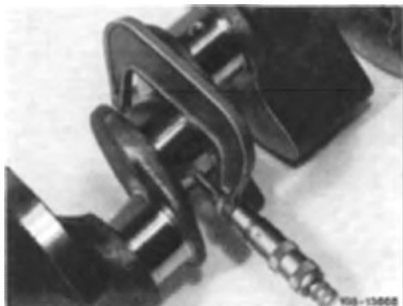
7 Measure width of fitted bearing journal and use pertinent thrust washers (refer to table, section "Data").
