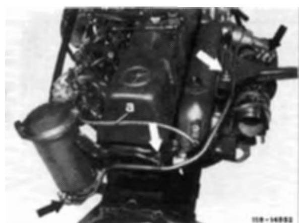
7 Unscrew supporting bracket for exhaust manifold on engine carrier.
