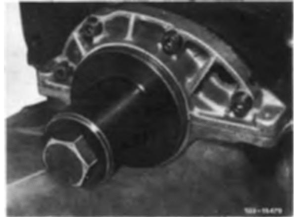
8 Install balancing disc, vibration damper and pulley (03-340).
