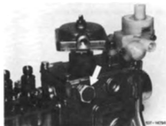
10 Check whether connecting rod (5) is correctly set, moving control lever (1) to full-load stop (2) for this purpose. Operating lever (8) must have approx. 0.5 mm clearance from full-load stop (6).
