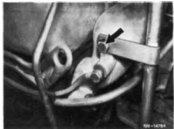
6 Loosen engine oil line (arrow) on oil filter and fastening clamp for engine oil line on cylinder head. On model 126, remove center part of partition for better access.
