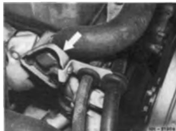
7 Unscrew closing plug of chain tensioner.
