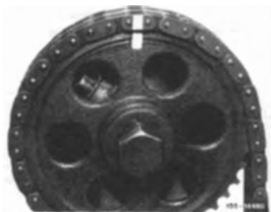
13 Remove camshaft sprocket.
