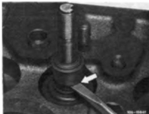
4 Lubricate new valve stem seals and mount by means of assembly mandrel.
