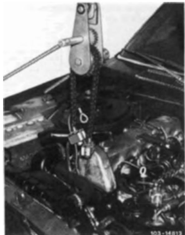
To remove oil pan, turn crankshaft with tool combination until oil pan upper half can be pulled past connecting rod or crankshaft webs.
