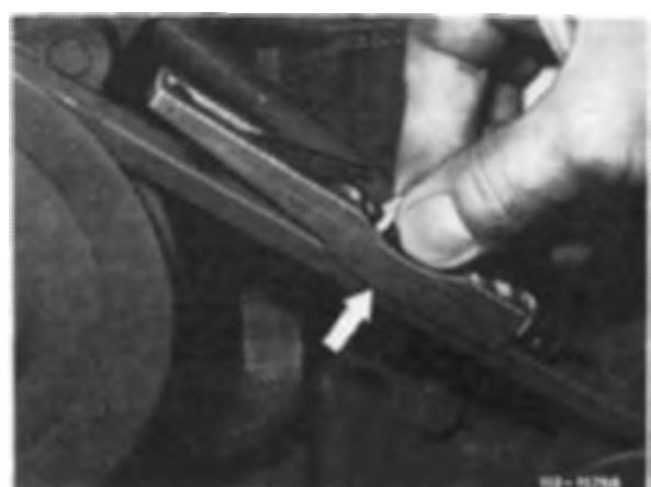
3 Exert a uniform, vertical pressure on V-belt upper surface by means of pushbutton, until click spring is audibly (or noticeably) disengaging.
