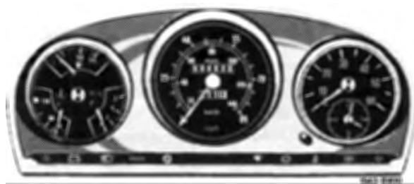
As soon as the required glow period, depending on coolant temperature, is attained, the preglow indicator lamp goes out and thereby indicates ready-to-start condition.
