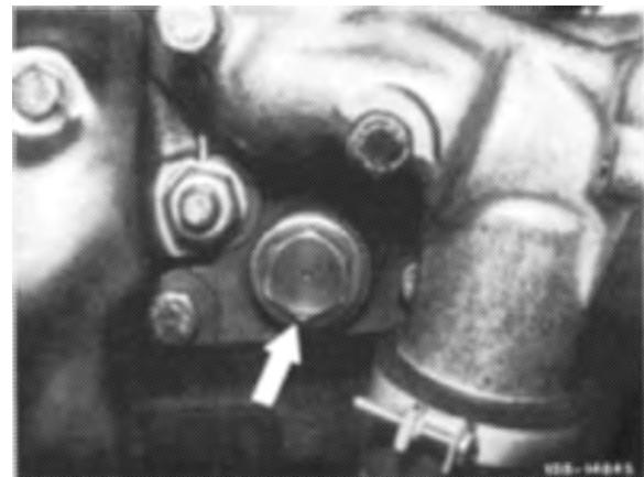
6 Remove compression spring in chain tensioner.
