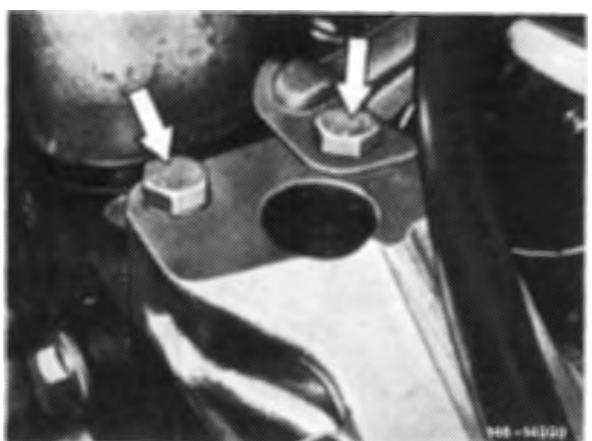
20 Remove cylinder head cover. For this purpose, disconnect regulating linkage. Pull out locking eye of longitudinal regulating shaft (arrow).
