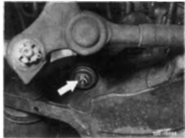
9 Loosen exhaust lateral support on transmission.
