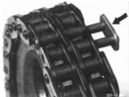
**Note:** Insert new connecting link from the rear so that the lock washers can be seen from the front (arrows).
