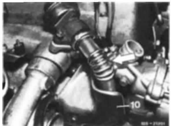
10 Unscrew closing plug of chain tensioner and remove compression spring (05-310).
