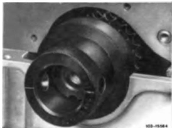
6 Coat all sealing surfaces with sealing compound, part no. 001 989 46 20.
