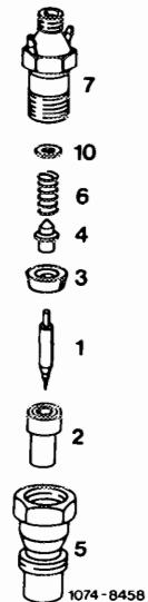
12 Clamp upper part (7) of injection nozzle in vise and torque lower part (5) to 70–80 Nm.
