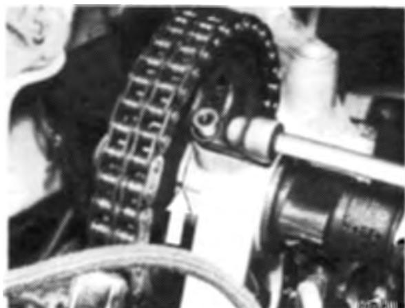
7 Using ink or paint, mark meshing point of chain on injection timing device, and position of injection timing device relative to crankcase.
