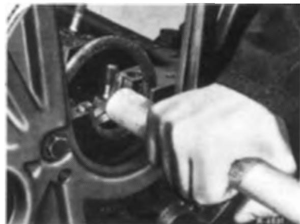
10 Provide thrust washers with engine oil and slip into grooves on fitted bearing (cylinder crankcase).
