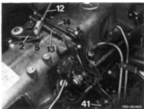
13 Check full load stop. With engine stopped, push accelerator pedal from inside vehicle up to stop on kickdown switch. Accelerator pedal and regulating lever on injection pump should rest against full load stop. If required, loosen adjusting screw (arrow). Adjust throttle linkage in such a manner that the regulating lever rests against full load stop.
