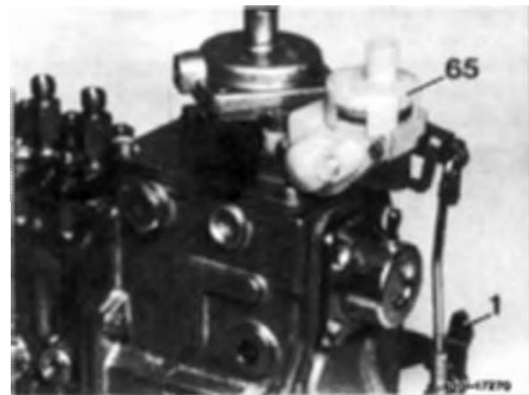
After bridging the idle path, the vent cross section in vacuum control valve is constantly increased under the increasing load and the vacuum is therefore continuously reduced. Venting proceeds via black plastic line (arrow) leading into passenger compartment.
