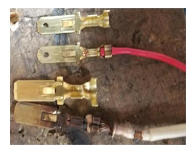
Connect the RED, BLUE, and BROWN wires with crimp connectors to the RED, BLUE, and BROWN wires coming out of the GPR harness.
